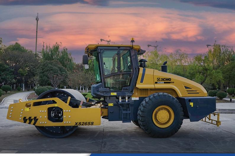
WEIGHT - 26000 KG GRADEABILITY - 50% DIMENSIONS (L\*W\*H\*) - 6990 x 2470 x 3430 mm STATIC LINEAR PRESSURE - 784 N/cm
