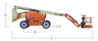
Platform Width 36-in / 0.91-m A. Platform Length 96-in / 2.44-m B. Machine Width 8-ft 2.2-in / 2.49-m D. Tailswing Zero Machine Height 8-ft 5.5-in / 2.58-m E. Machine Length 30-ft / 9.14-m Wheelbase 8-ft 1.9-in / 2.48-m
