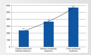
Medium hardening treatment, steel hardness can be increased by 55% on the basis of the original metal base material hardness; Extra hardening treatment, steel hardness can be increased by 140% on the basis of the original metal base material hardness, which is suitable for vibration wheels under severe working conditions.
