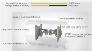
Durable full-fusion reinforced drum; XCMG special long-life vibration bearings, the theoretical life of up to 10,000h.
