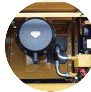
Air filter maintenance space
