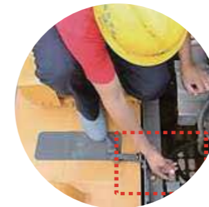
Pump oil by one push after engine goes off abnormally
