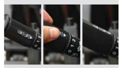
Three forward gears - Suspension hydraulic transmission with three forward gears, top speed reach 25km/h.
