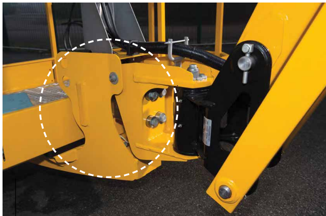
LOAD SENSING SYSTEM PROTECTED within the platform yoke assembly
