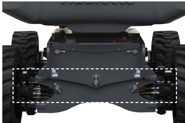
STEERING CYLINDERS PROTECTED inside the frame
