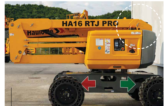
BOOM PROTECTED by the counterweight frame
