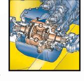
truck is travelling, thereby boosting productivity. In addition, the differential lock switch, which is a three position switch, can lock up the rear axle differentials only, or all axles for maximum performance in the worst conditions.
