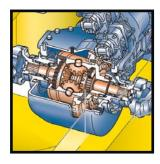
In addition, limited slip differentials prevent the tires on either side from slipping on soft ground.
