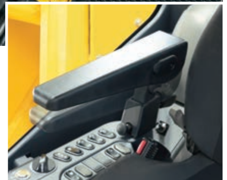
Armrest with simple height adjustment
