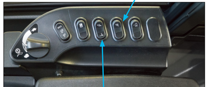
Attachment selector switch
