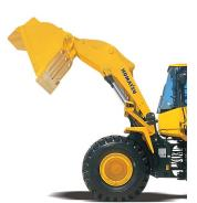
The long lift arms provide high dumping clearances and maximum dumping reach. The operator can even level loads on the body of a dump truck easily and efficiently.
