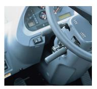
Easy shifting and directional changes with Komatsu two-lever electronic shifting. Change direction or shift gears with a touch of the fingers without removing the shifting hand from the steering
