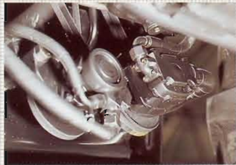
The independent high capacity hydraulic pump supplies 40 l/min and is readily accessible for servicing.
