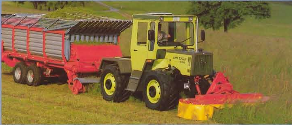
With a front mower and self-loading trailer, the MB-trac becomes a „fodder express“ – a classic combination for zero grazing or one man silage harvesting.
