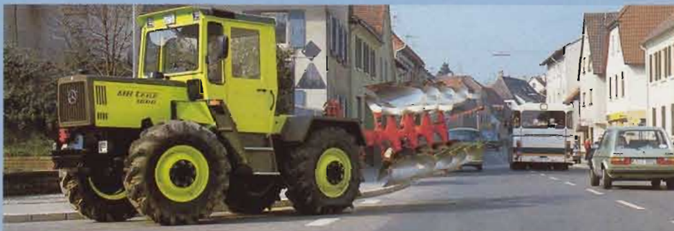
With 4 wheel brakes, front sprung axle and plenty of front end weight, the MB-trac can be driven on public roads with heavy fully mounted ploughs with complete safety.
