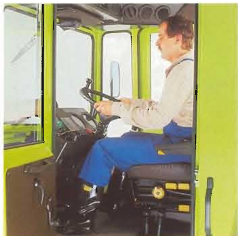
The comfortable seat which is equipped with spring suspension and hydraulic damping is adjustable to suit each driver, tilting of arm rests, back rest and seat cushions, as well as seat height and fore and aft adjustment.
