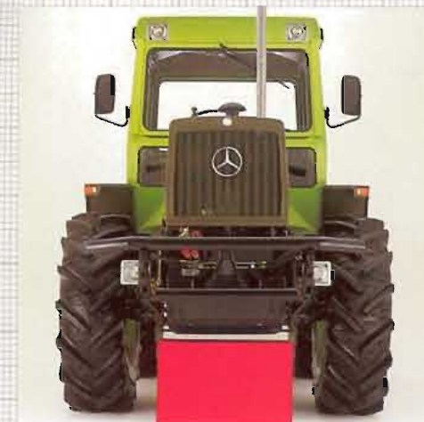
The hub-reduction axles provide high ground clearance, essential for row crop work.
