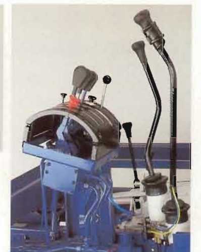
Ideally spaced gear ratios and synchromesh, even when changing from forward to reverse.
