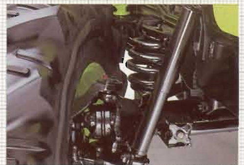
The sprung front axle absorbs severe bumps and the shock absorbers prevent bounce. With such suspension there is also more lateral support, making it safer when crossing hillsides than with a conventional centre pivot axle.
