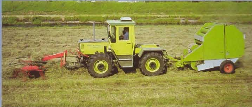
With front mounted swathers, the windrow is not driven over, thus giving a cleaner pickup; windrowing does not get ahead of the baler and two jobs are done in one pass.
