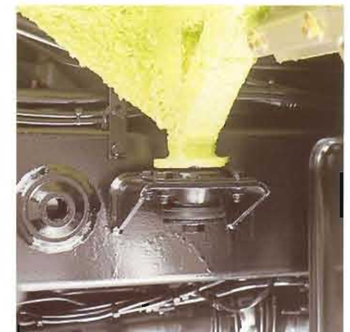
The three resilient cab mounts, on special vibration dampers, contribute considerably to the driving comfort.
