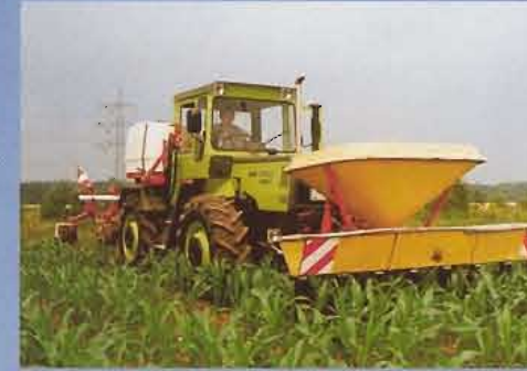
Mineral and liquid fertilizer application combined with inter-row cultivation.
