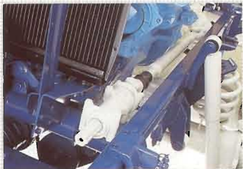
Full engine power can be taken at the front as well as at rear or at both P.T.O.'s simultaneously with a choice of 540 or 1000 rpm.
