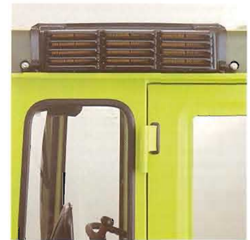
Large filters ensure that the three-stage fan delivers dust-free air. Air conditioner is optional.
