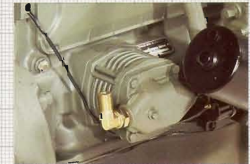
The maintenance-free and reliable engine-mounted compressor provides auxiliary power for the braking system.
