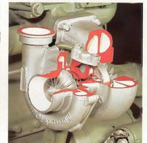
The OM 314 A's turbocharger provides more air, more oxygen and excellent fuel economy.
