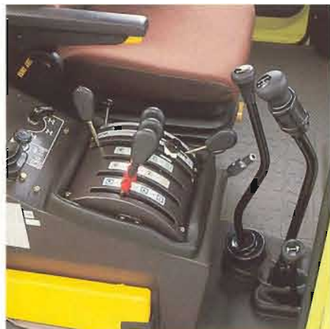
The control levers for the transmission, hydraulic system, all-wheel drive and differential locks are on the right next to the driver's seat.
