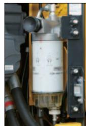
Removes water and contaminants in the fuel to prevent fuel problems.
