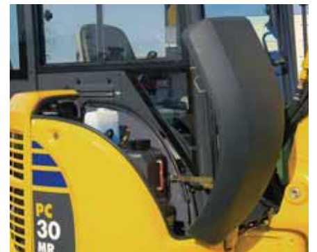
Front bonnet: fuel tank refilling
