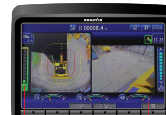
Ecology gauge Fuel consumption gauge
