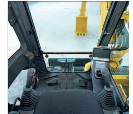
Lever shown in lock position
