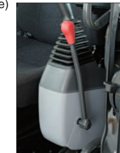
Lever shown in lock position
