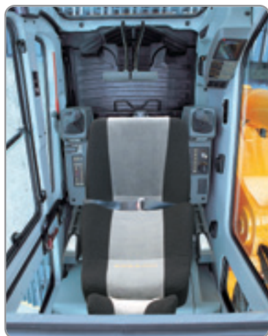
1 2 3 ① Wide, Comfortable Operating Space ② Steel Cover Sunroof ③ Dial Type Engine Speed Switch and Key Switch
