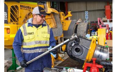
Major component overhauls on all parts including transmissions, engines, diffs, and undercarriages.
