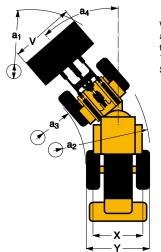
Where applicable, specifications and dimensions are according to ISO 7131, SAE J732, ISO 7546, SAE J742, ISO 14397, SAE J818.
