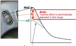
S-mode: Improve tire slip ratio on snowy or slippery road condition
