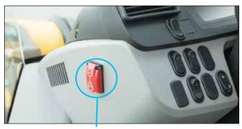
Engine shutdown secondary switch
