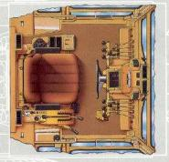
■ Electronic Monitoring System (EMS) — shows status of important machine systems. Operator concentrates on production instead of watching gauges. Reduces the possibility of catastrophic failures and subsequent costly repairs.
